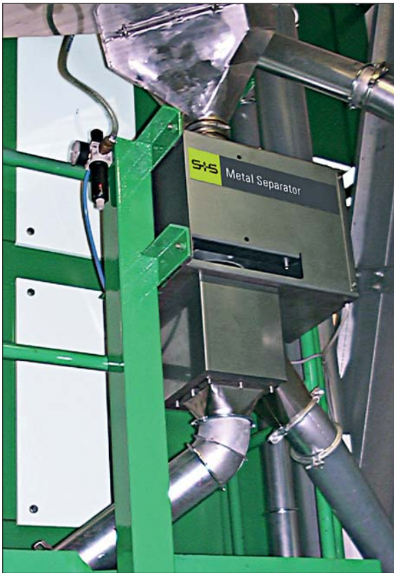
Metal separator RAPID 4000-FS used for quality control at a filling station for dried vegetable.
