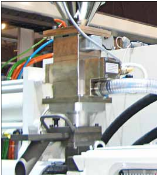
PROTECTOR PRIMUS metal separator installed at the material infeed of an injection moulding machine
